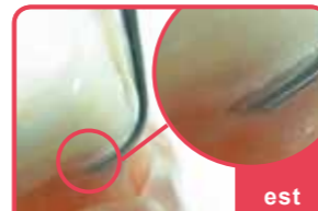
est It becomes much easier to control just by designing the blade slightly shorter.
