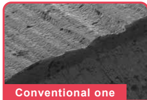
Conventional one Blade surface is not smooth enough due to conventional sharpening process. So it's easier to be dull than "est" series.
